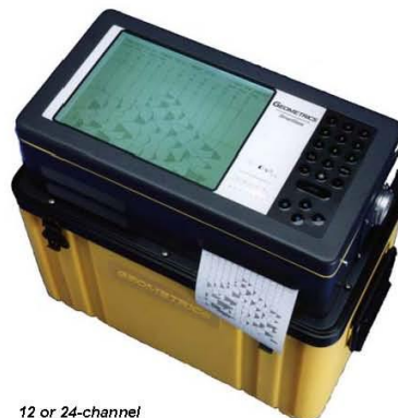
12 or 24-channel exploration seismograph
